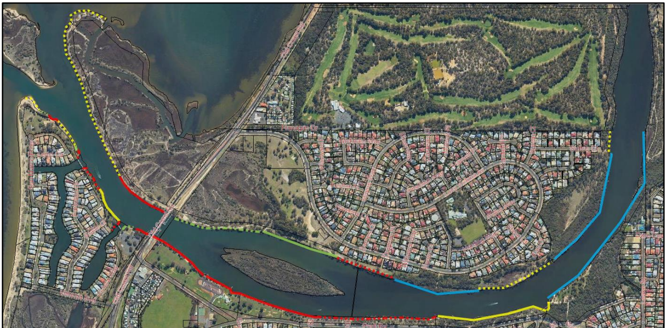
Figure 3-8 Priority of Foreshore Erosion Control (Image source: DWER 2018). Red = priority 1 (0-5 years), Yellow = priority 2 (5-10 years), Green = priority 3 (Greater than 10 years), Blue = no works required
