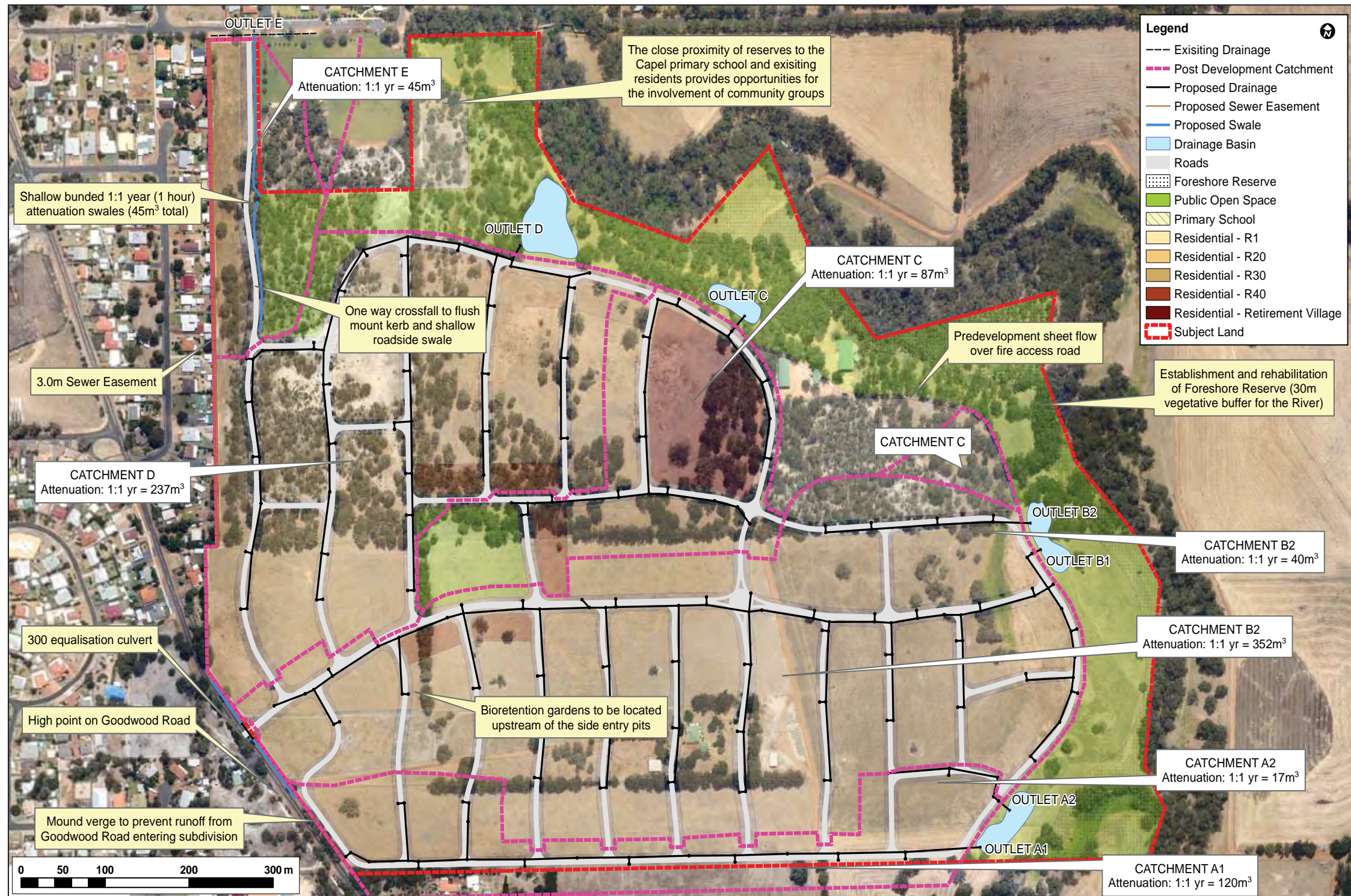
Figure 11 - Drainage Management - 1:1 ARI Event
