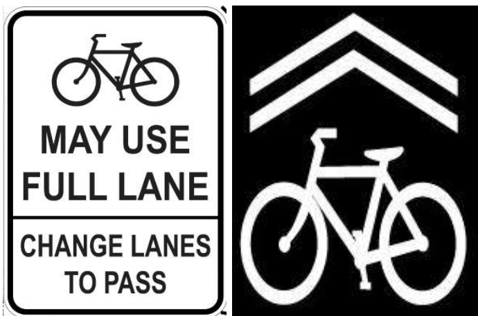
Figure 2-6 On-Street Mixed Traffic Cycling Signage and Linemarking
